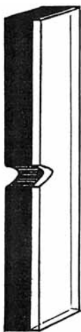
Fig. 1. Brittle-layer impact specimen. The 0.020-in. brittle layer is shown on the right-hand side.
